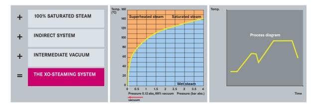
The XO-Process for vacuum-steaming of textiles uses 100% saturated steam and the renowned XO-Intermediate Vacuum Procedure. This is a prerequisite to guarantee even treatment of the textile material and to assure the correctness of the process.
